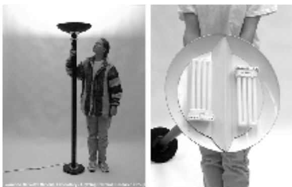
Figure 1: Example of CFL Torchiere being used at Stanford University test site. The luminaires are similar in look to halogen torchieres, but they use 2 fluorescent lamps in a white reflector dish (as seen on right).
