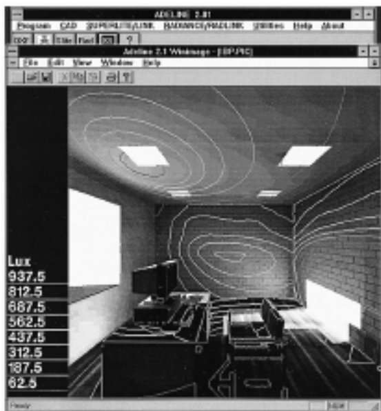
Figure 2. ADELINE graphical user interface under Windows NT. The image background shows the ADELINE main menu, the front shows a photorealistic visualisation generated with RADIANCE NT, displayed from within the ADELINE GUI.
